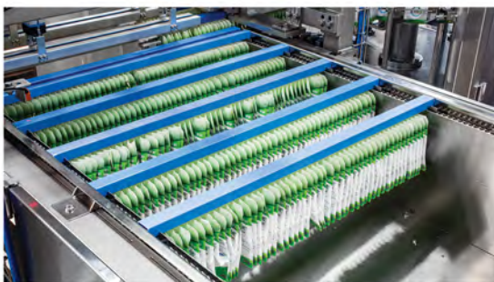
Pre-Made Top Spout Pouch fed via pre-loaded rail system
