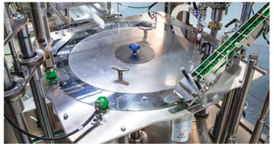
Rotary carrier filling star wheel
