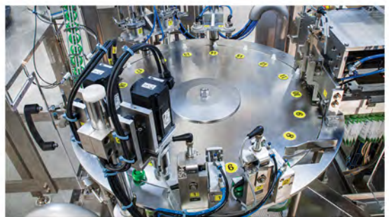
Rotary carrier filling star wheel
